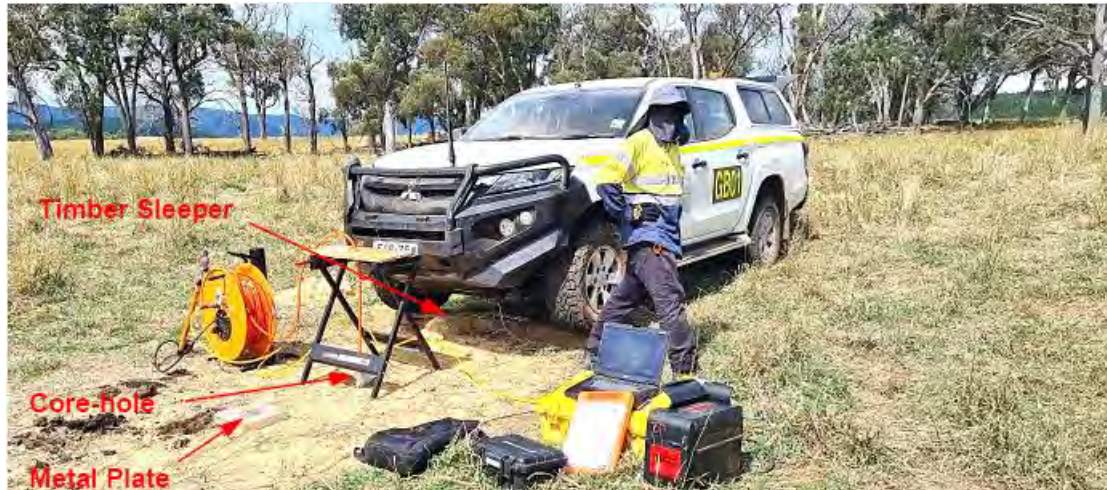
Figure 2: A typical VSP field equipment set up
