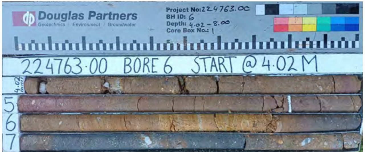
Bore 6 – 4.02 m to 8.0 m
