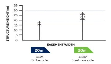
**66kV single pole structures,** which reside in a typical 20m wide corridor, would be replaced by one new steel monopole one of two arrangements, either: 132kV steel monopole (above left); or 132kV with 66kV underbuilt steel monopole (above right).
